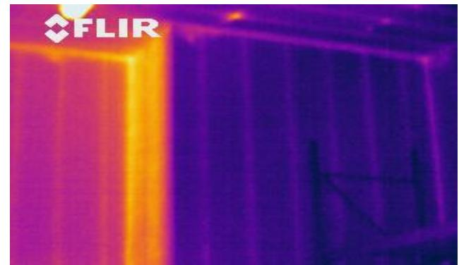
The missing freezer ceiling sections of insulation, from inside the freezers. Yellow areas are voids.
