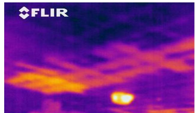
The missing freezer ceiling sections of insulation, from outside of the freezers. Blue areas are voids.
