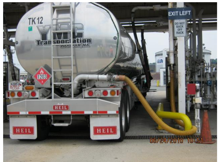
2. Tank Truck in loading bay receiving product.
